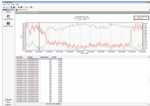
Counter report: The electricity consumption (active power) and the according power factor (cos phi) are reported in 15 min. interval. During weekend fewer machines are in production. As a result the active power decreases and the power factor improves. The graph shows that the power factor always remains above 0,9, which indicates an acceptable situation. This graph also allows to evaluate the functioning of the condenser battery for improvement of the power factor.
